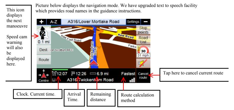
Unlike other navigation systems, Navigation Master 'Cabbie's Mate' has been designed to be scrolled instantly. The map is best scrolled using either the back of your nail or the stylus supplied with the unit, when you have finished scrolling tap on 'Centre' icon for your current position. Our new design has reduced screen tapping compared to other systems.
